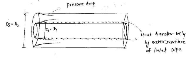
$$\left(\begin{array}{ccc} \text{Deq} & = & 4 & \frac{A}{P} \end{array}\right)$$
